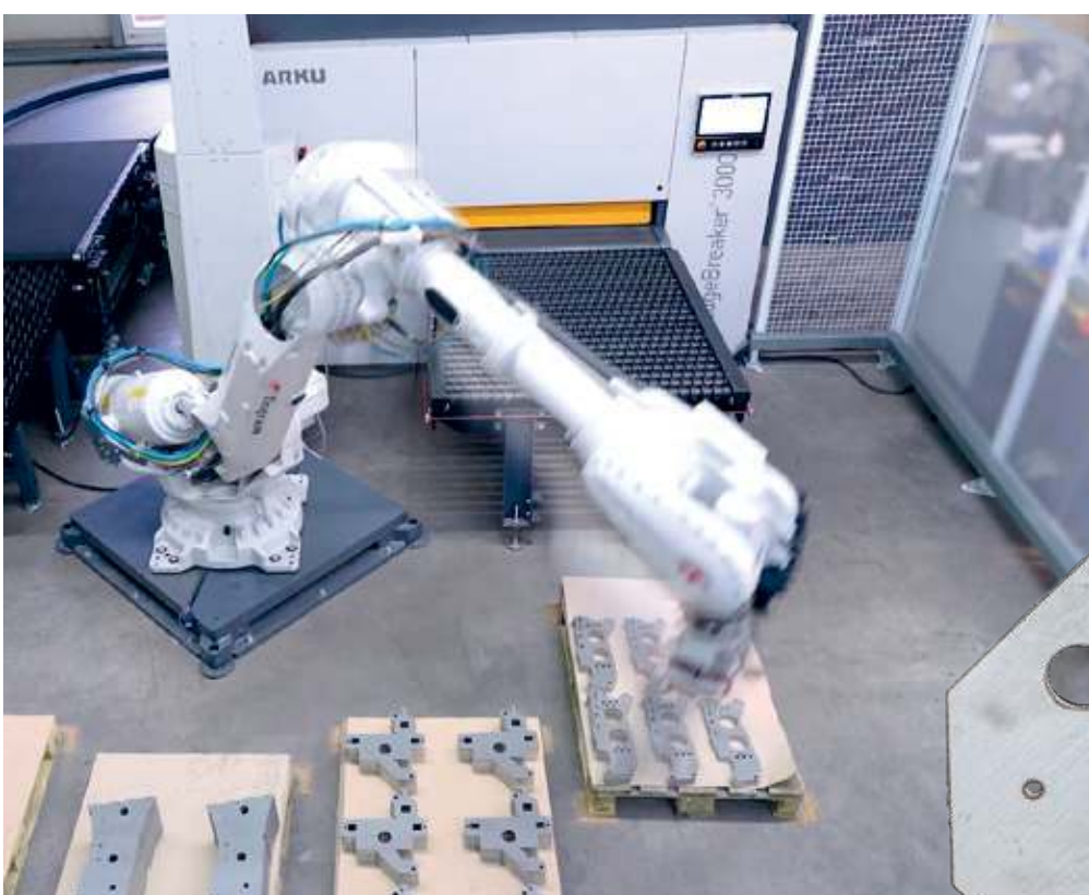
Intelligent automation in action: The robot takes over the precise deburring of components - efficient, repeatable, and around the clock.
