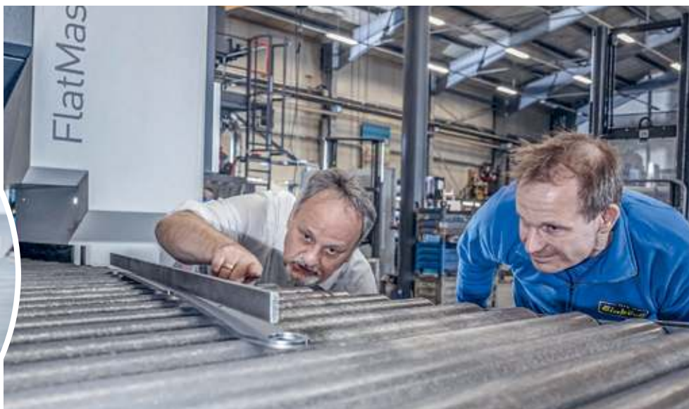
A closer look before the first step (left to right): Thomas Weinfurtner, Sales at ARKU, and Robert Clemens, an Einböck employee, inspect the sheet metal before processing and define the required leveling specifications.
