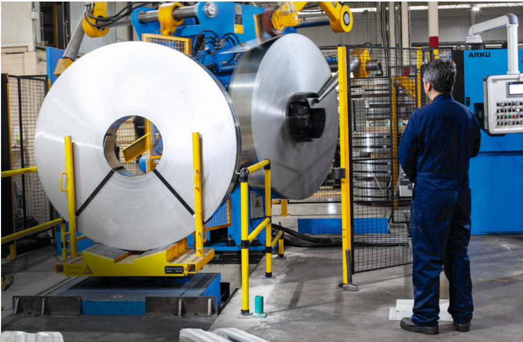
Speed is key: thanks to the double-sided decoiler on the new ARKU line, employees can ensure production has no downtimes to keep up with demand.
