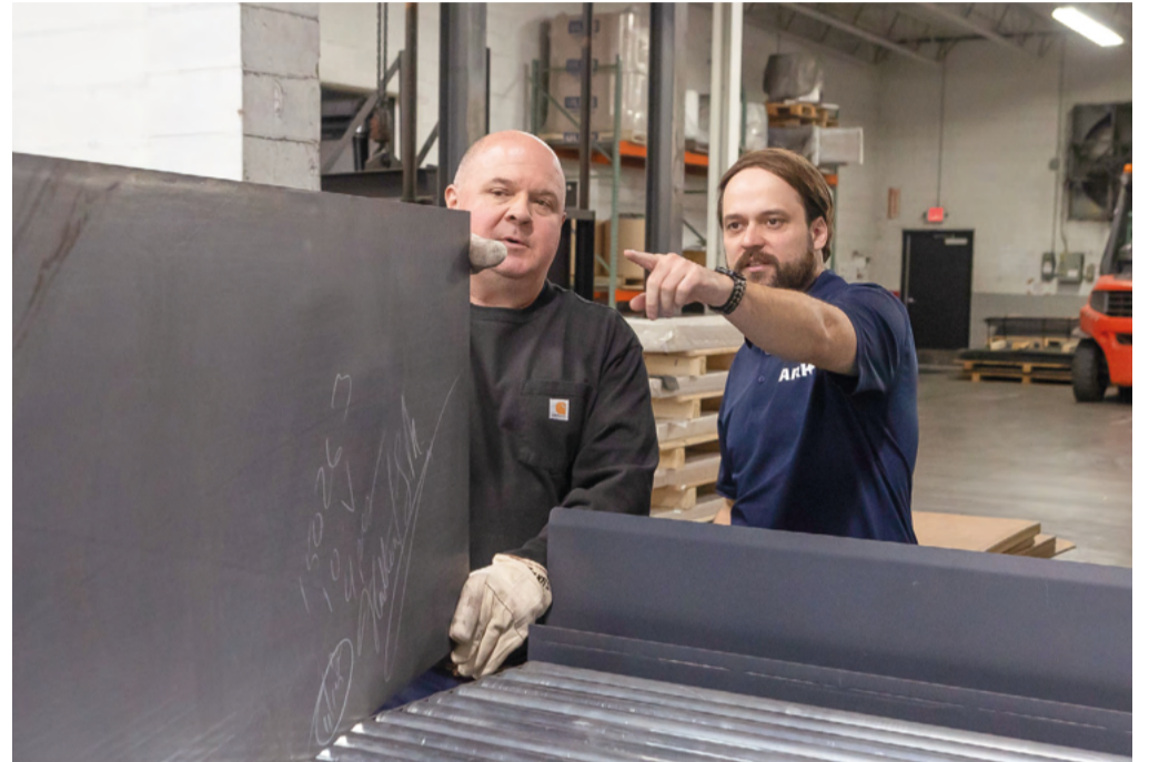
Bill Gross and Denis Weinfurtner are examining a piece of metal after the leveling process to see if all flatness deformities have been removed.
