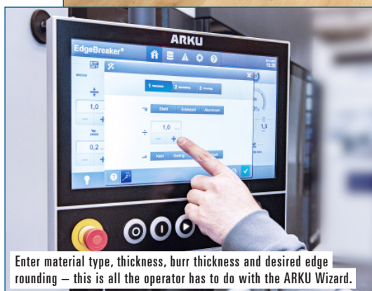
ISMR watched a demonstration on ARKU's EdgeBreaker® 6000 deburring system.
