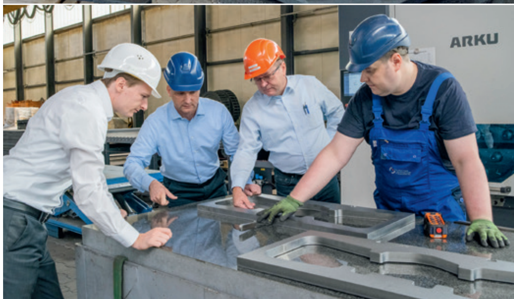
Hard facts: from left to right Christian Nau, Sales at ARKU, Daniel Götze, Product Manager Pre-processing at SMSD, Norbert Gärtner, Plant Manager at SMSD, and Patrick Völpert, Machine Operator at SMSD, check the flatness of the leveled parts.
