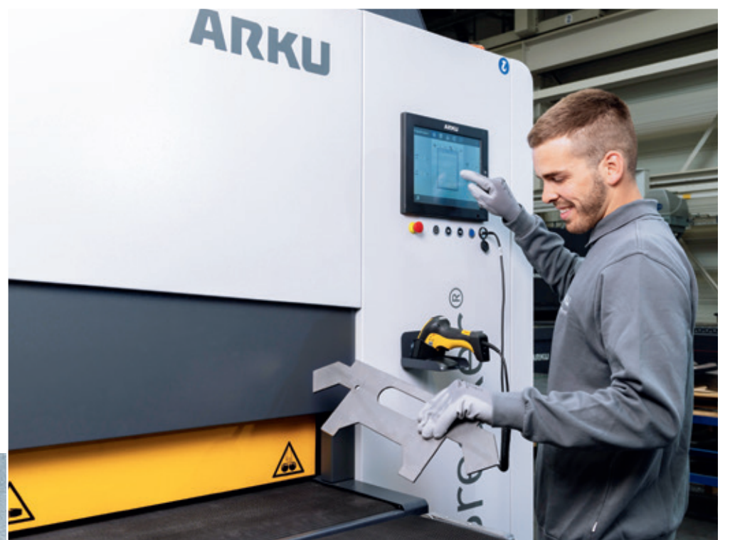
Double-sided deburring and edge-rounding for laser-cut parts in one process with the EdgeBreaker® 3000.
