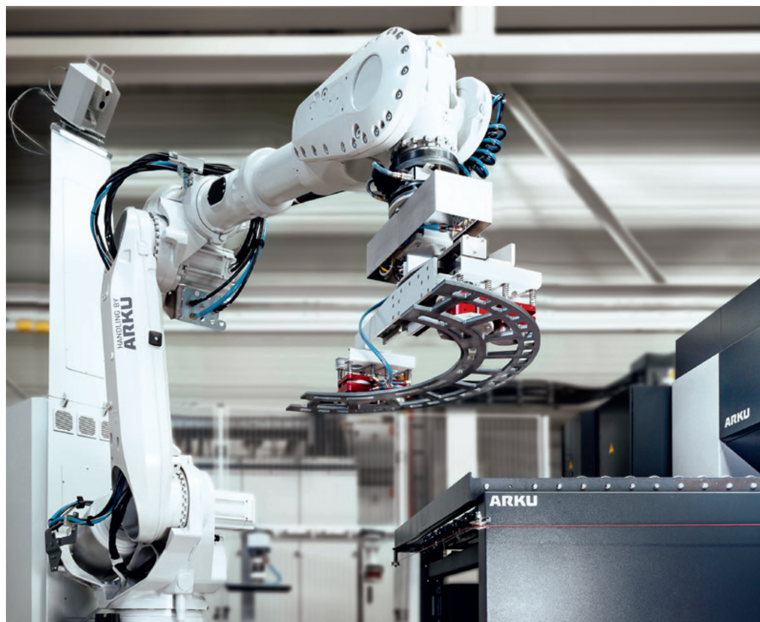
A reliable worker: The Vision robot lifts the parts and places them precisely on the roller conveyor of the FlatMaster 88®. The leveling process can start immediately, without any additional manual correction.
