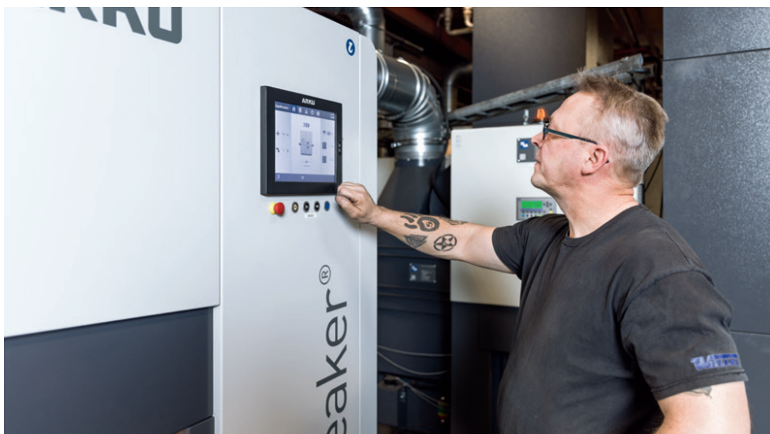
Weland utilizes the EdgeBreaker® 4400 deburring machine to deburr and round components up to 100 mm thick on one or both sides.
