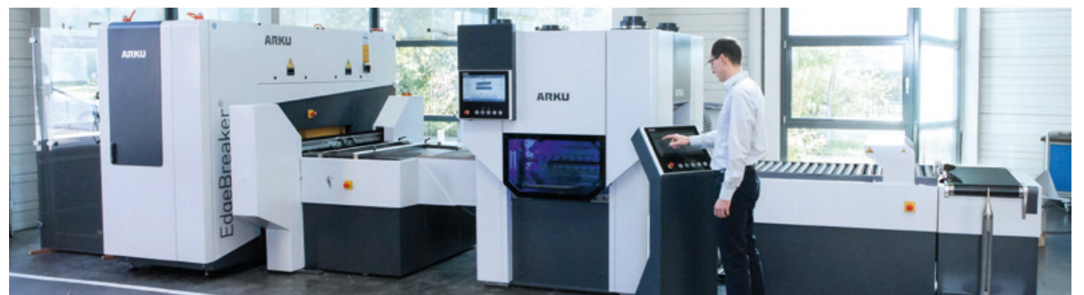
The process chain at a glance: deburring with the EdgeBreaker® 2000 Plus, leveling with the FlatMaster® 55 80 and flatness control with the FlatJack® in a line.
