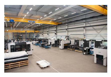
ARKU deburring and leveling machines are being assembled in Bühl.
