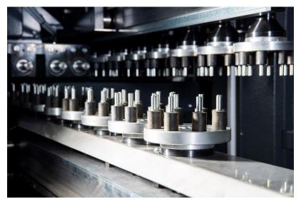
Caption: These tools outfitted with pins in the EdgeBreaker® 5000 remove slag from the cut parts.
