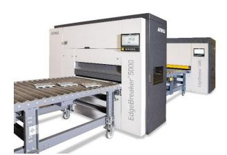
Caption: Two becomes one: The new EdgeBreaker® 9000 Line combines the EdgeBreaker® 5000 slag hammer with the EdgeBreaker® 4000 deburring machine.
