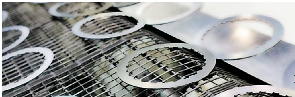
Maintaining extreme flatness is mission-critical for transmission components to ensure smooth shifting from gear to gear.
