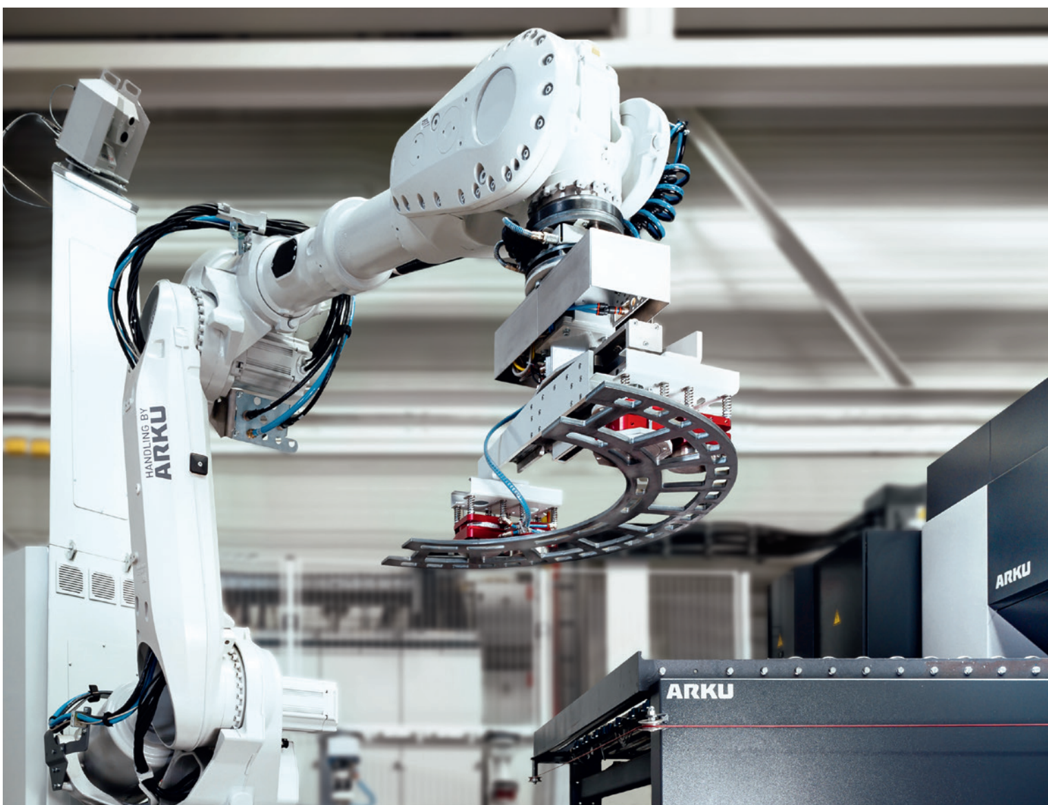
A reliable worker: The Vision robot lifts the parts and places them precisely on the roller conveyor of the FlatMaster 88®. The leveling process can start immediately, without any additional manual correction.
