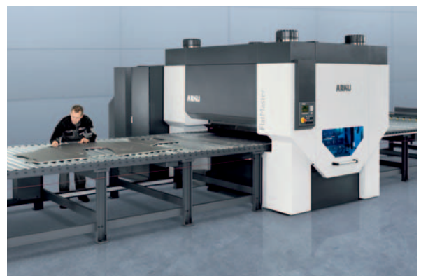
Precision levelers like the Arku FlatMaster provide better leveling results in just a few minutes – even for thick flame-cut parts
