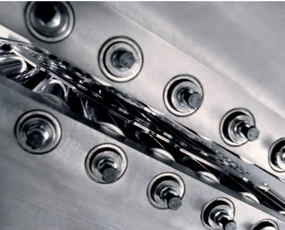
A closer look at a leveling unit where the parts are deformed by alternate bends to get them flat and stress-free
