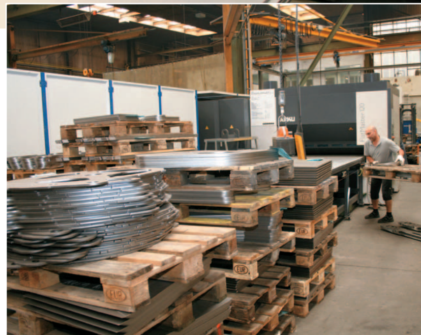
The FlatMaster® 120 provides best leveling results for many different laser- and flame-cut parts at Liebherr
